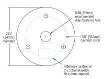
NOTE: #6 [3.5mm] flat head or oval head screws are recommended for installation.
